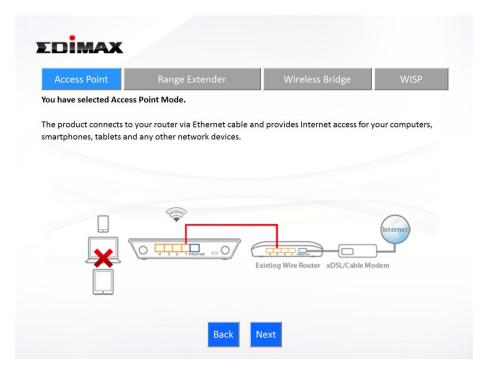
**2.** Connect the LAN port of your BR-6428nS V4 to the LAN port of your existing router using an Ethernet cable, then click "Next".
