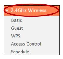
The "2.4GHz Wireless" menu allows you to configure SSID and security settings for your Wi-Fi network along with a guest Wi-Fi network. WPS, access control and scheduling functions can also be managed from here.
