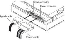
Figure 3. Attaching SATA cabling
