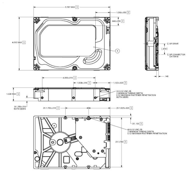
Figure 4. Mounting dimensions—top, side and end view
