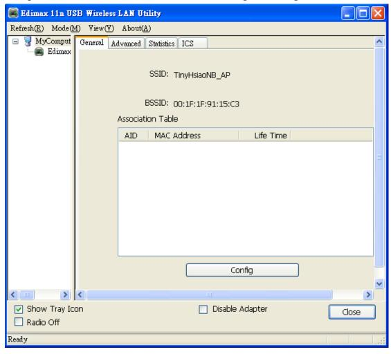
After mode switch is complete, you'll see general information of software AP, which shows AP's SSID and connected wireless clients.
