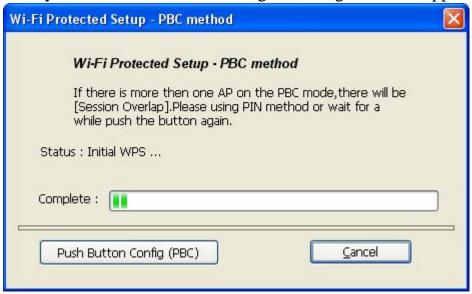
Please activate Push-Button function on wireless access point now, and wireless network card will establish secure connection with access point within one minute.
